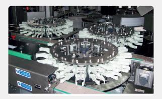
Advanced starwheel clamping system: one star fits all bottle types and sizes, so no additional format changeover time is required.
