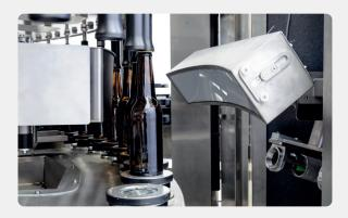
High quality labeling, accuracy and efficiency guaranteed by precise positioning thanks to the fully automatic optical bottle orientation system.
